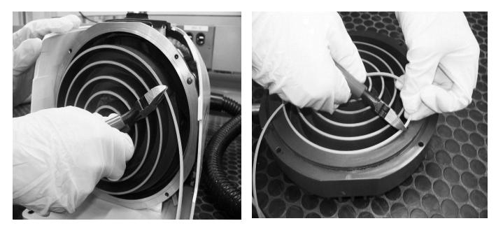
12. Lightly lubricate the new main O-ring with a trace amount of Krytox LVP grease provided and install into the O-ring groove.
