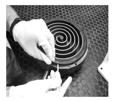
7. Remove the old tip seals from both the outboard housing and orbiting plate.
