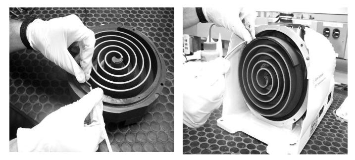
8. Clean all debris from both the outboard housing and orbiting plate surfaces (including the O-ring groove and tip seal grooves). Use isopropyl alcohol and a scour pad (preferably non-scratch) to remove any buildup on all surfaces. Wipe clean with a low-lint or lint-free cloth and cleaning swabs.
