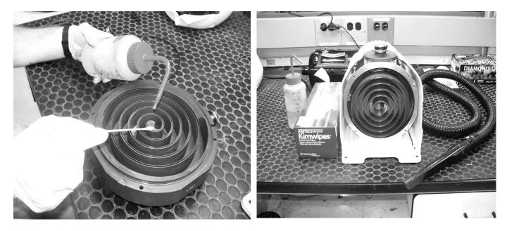
9. To install the new tip seals, start from the center of the scroll, leaving a 1/8<sup>th-</sup>inch or 3 mm gap at the center (as shown).
