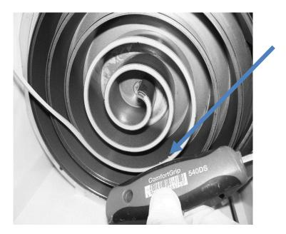
11. Finish installing the rest of the tip seal and using a set of cutting pliers, cut the tip seal leaving a  $1/8^{"}$  inch or 3 mm gap from the end of the tip seal groove (as shown).
