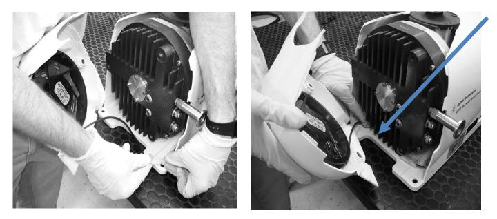
15. Reinstall the fan cowling and the three M6 screws onto the pump. Ensure that the points of the cowling are properly sitting on top of the cover plate tabs.
